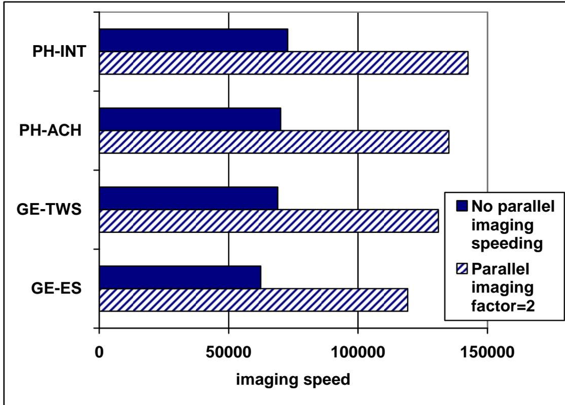
Graph 17. Comparison of 2D imaging speed with EPI-type sequences (pre-scan separate from main scan)
