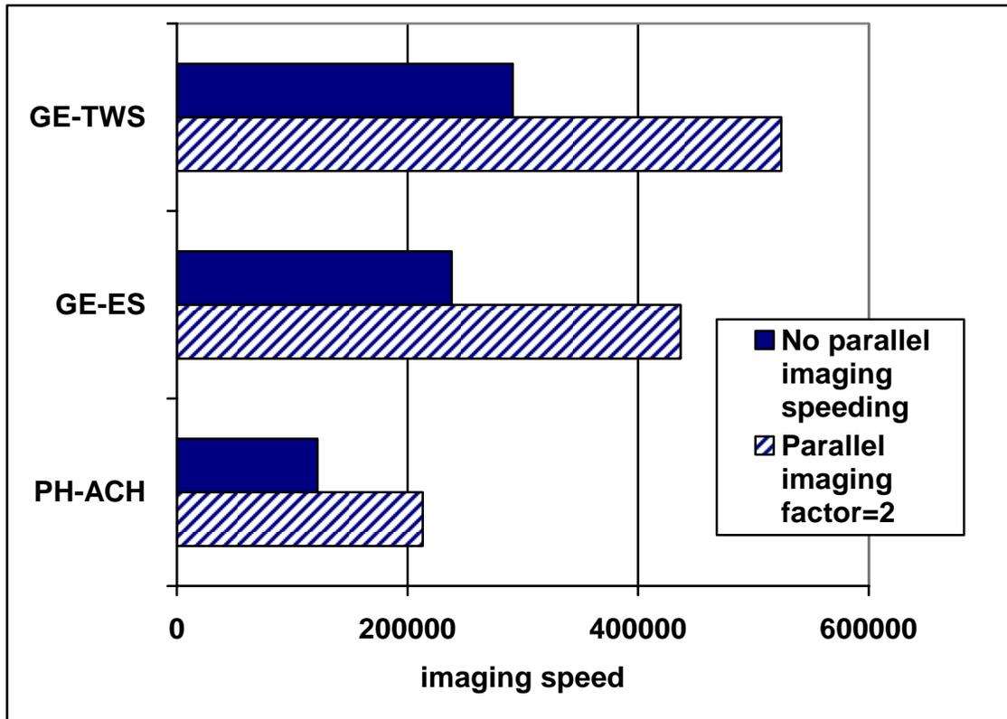
Graph 18. Comparison of 2D imaging speed with EPI-type sequences (pre-scan included in main scan)
