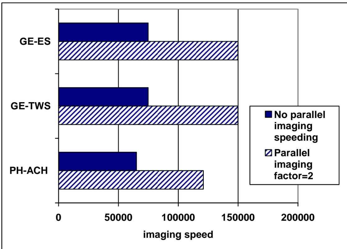
Graph 20. Comparison of 3D imaging speed with GRE-type sequences
