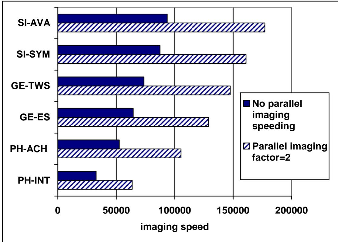
Graph 21. Comparison of 3D imaging speed with FSE-type sequences
